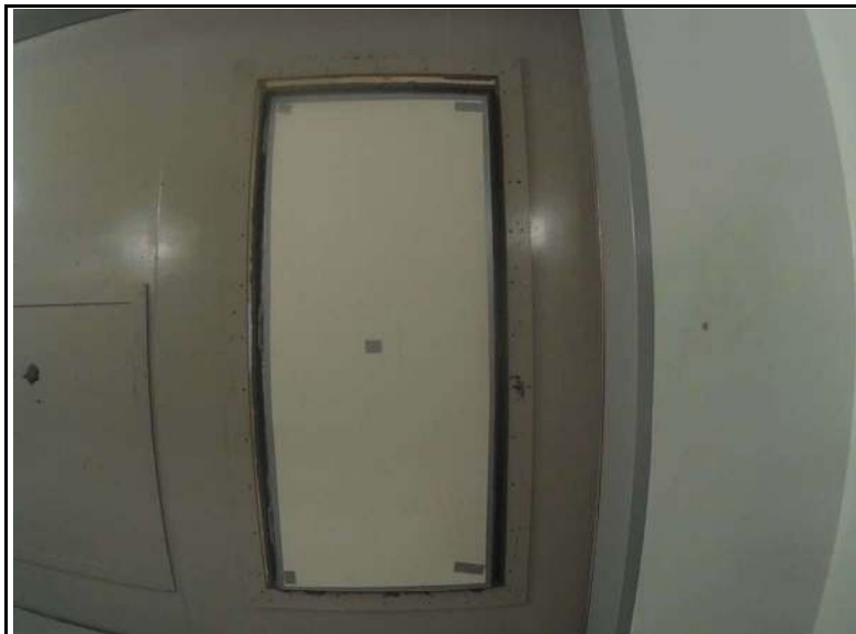
Receive Room View of Test Specimen
